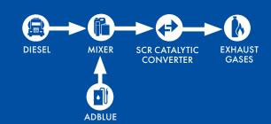
Most vehicles are typically fitted with a 70 or 150 litre tank and will need to be topped-up with AdBlue every two to three tanks of fuel. It is recommended that the vehicle carry a reserve supply of AdBlue to ensure the vehicle fitted with a SCR system will perform at its maximum efficiency. AdBlue is non-toxic and poses no risk, if properly handled, to the environment, animals or humans.
